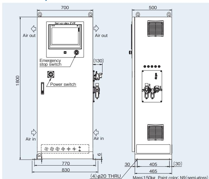
\* The control panel size varies, depending on the motor size and type.
