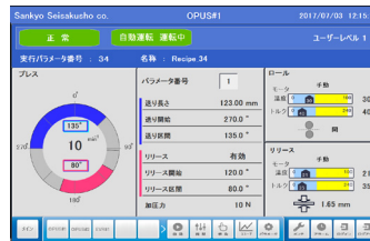
Automatic operation screen
